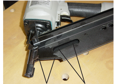
Probe in these areas with a screwdriver to release jammed nails.
