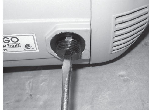
Inspecting the Carbon Brushes (50)
