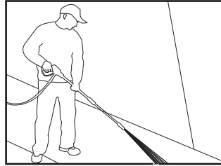
Figure 5 Optimum angle to cleaning surface
