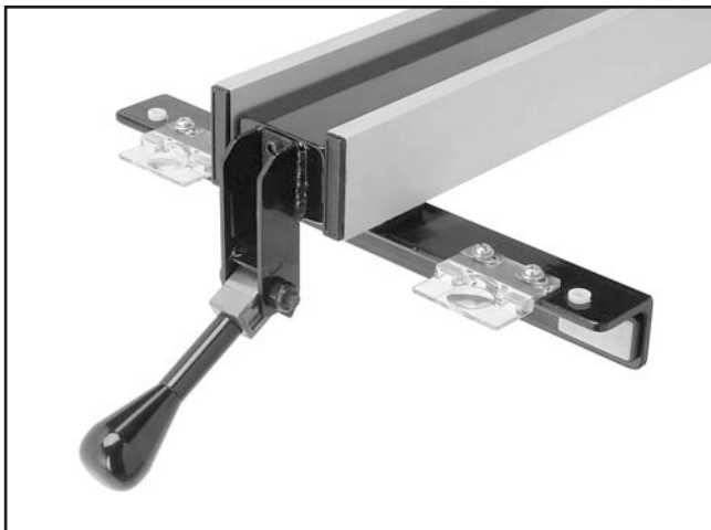
Figure 32. Fence knob installed.
