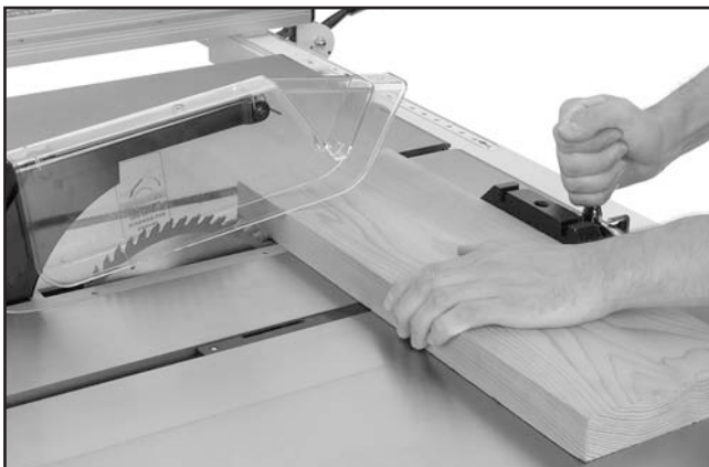
Figure 44. Typical crosscutting operation.
