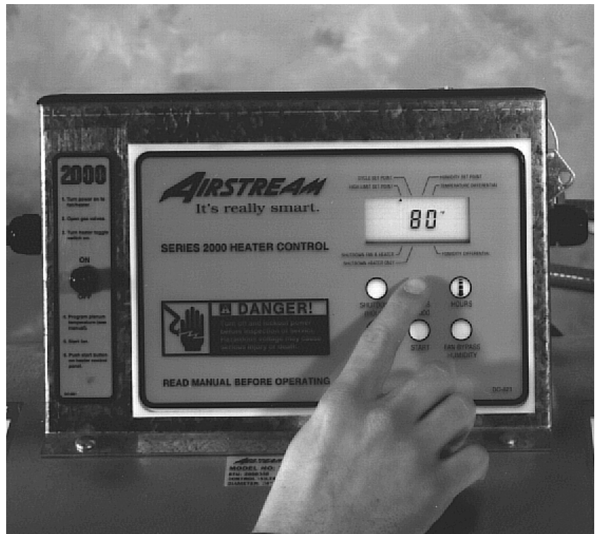
Programming the high-limit set point.
