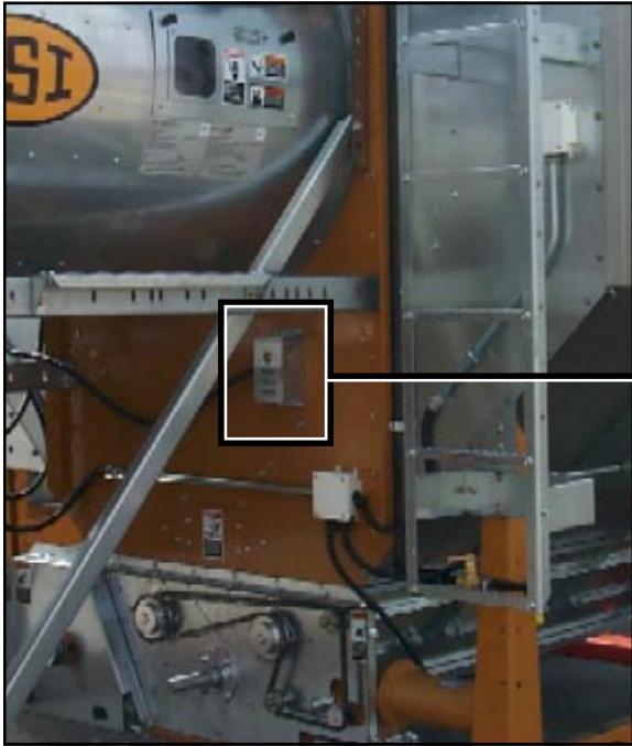
Air Switch location.
