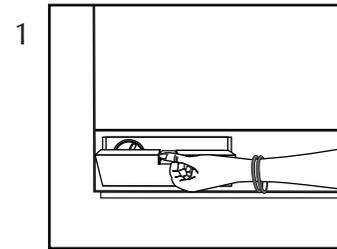
Open the bottom door, which is detachable by pressing the top portion of it.
