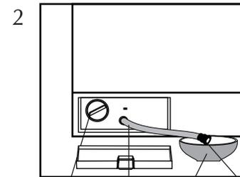
Place a shallow container near the bottom door. Pull out the drain hose and open the drain plug to drain out the water from the machine in the container.
