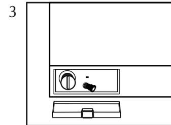
After draining out the water through the drain plug, open the coin trap by rotating in anticlockwise direction and remove the foreign particles like coins, pins, hooks, present if any. Tighten the coin trap and drain plug to their original positions and close the bottom door.
