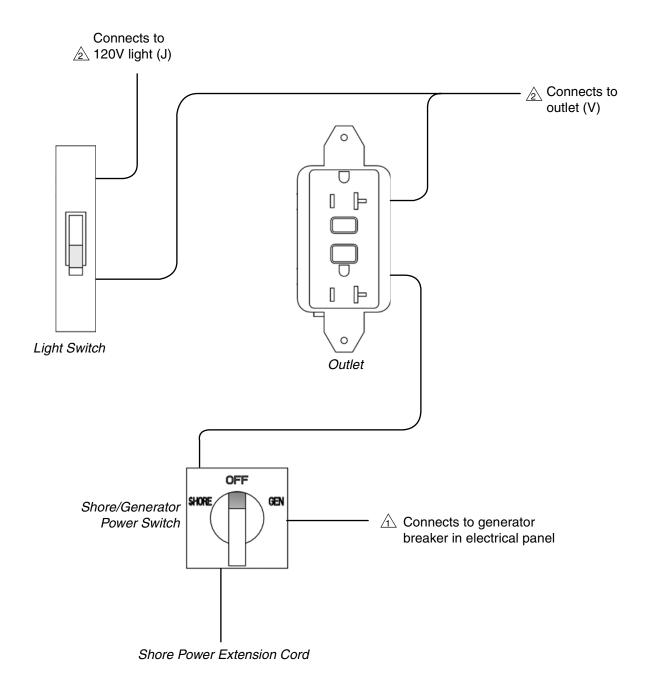
See Trailer wiring figure for your trailer configuration.
