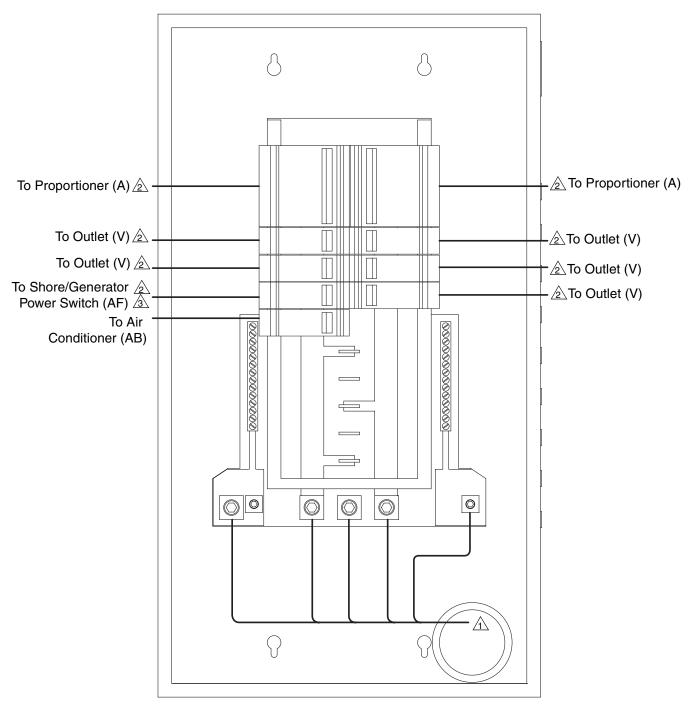
Connects to Main Breaker. See Main Breaker wiring, Fig. 18 on page 30.
