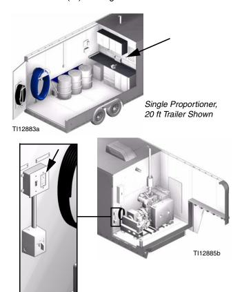
Fig. 9: Outlets Powered by Shore Power in 28 ft Trailers
