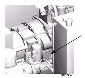
Fig. 7: Generator Grounding Point
