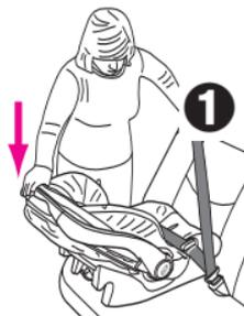
Holding the infant restraint ❷ or base ❸ near the vehicle belt path, TWIST AND PULL the infant restraint forward and to both sides to make sure the vehicle belt or **UAS** does not lengthen or loosen and the infant restraint does not easily move. The infant restraint should not move side to side or forward more than 2.5 cm (1 inch).
