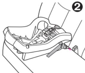
**Belt must lay flat and not be twisted.**
