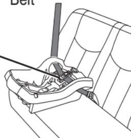
3. To create a secure installation, while pushing down on the base, pull the free end of the lap belt or the shoulder portion of the lap/shoulder belt to tighten ④.
