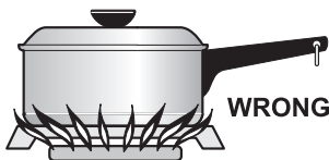
Improper Flame Size
