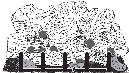
Figure 28 - Installing Scrap Log Pieces
