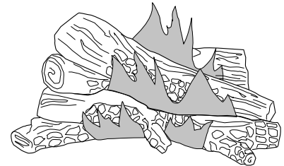
Figure 57 - Typical Flame Pattern for CHDV37N/P and CHDV41N/P
