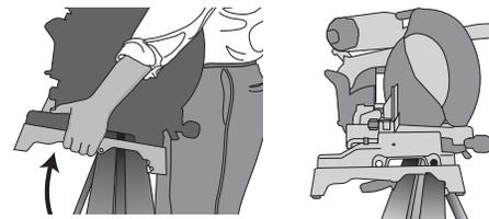
9. Approach the beam with saw/bracket assembly tilting toward your body slightly. Engage the concave front lip of the mounting bracket with rounded edge of beam. One of the brackets must engage the locator clip (G) to prohibit lateral movement of the saw during use.
