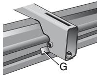
10. When front edge of the beam and locking locator clip are engaged, a slight downward pivot will allow secure engagement of the rear levers to back of beam. Rock the saw gently on the brackets to verify locking in position.
