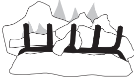
Figure 12 - Correct Burner Flame Pattern
