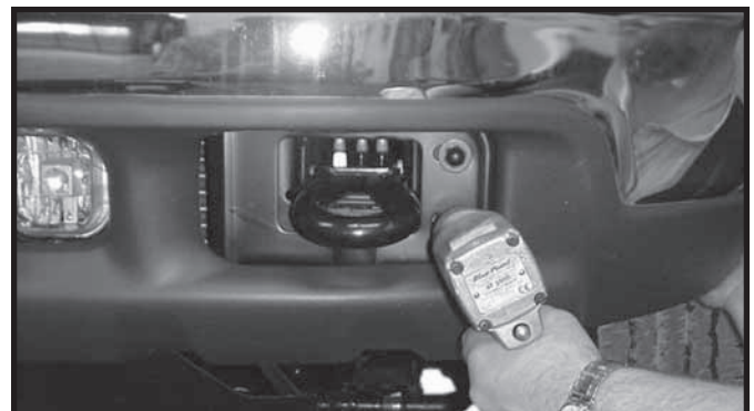
1b. On one side only, remove two bumper bolts on the front of bumper, out side of tow hook. These bolts will not be reused.
