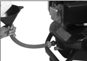
5. **Pull engine starter rope slowly several times** until antifreeze comes out of high pressure hose connection of pump.
