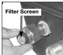
**NOTE:** Do not operate pressure washer without filter properly installed.
