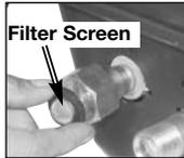
4. Connect water source to pump inlet. **NOTE: Water source must provide a minimum of 5 gallons per minute at 20 PSI.**
