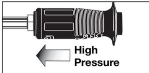
The nozzle at the end of the multi-adjustable spray wand can be rotated to change the high pressure spray pattern from a 0° pencil stream to a 40° fan spray, as shown. Markings have been placed on the nozzle to help you select the spray pattern.
