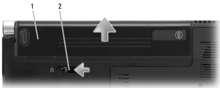
1 battery 2 battery release latch
