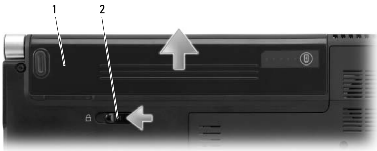
1 battery 2 battery release latch
