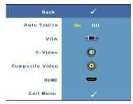
**AUTO SOURCE**—Select On (Default) to automatically detect the available input signals. When **On** is selected and you press Source on the control panel/remote, it automatically finds the next available input signal.
