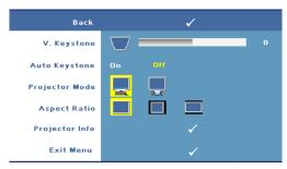
**V. KEYSTONE**—Allows you to adjust image distortion caused by tilting the projector.
