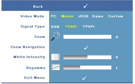
VIDEO MODE—Select a mode to optimize the display on how the projector is being used: PC, Movie, sRGB (provides more accurate color representation), Game, and Custom (set your preferred settings). If you adjust the settings for White Intensity or Degamma, the projector
