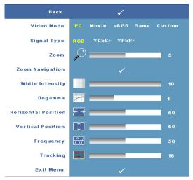
VIDEO MODE—Select a mode to optimize the display on how the projector is being used: PC, Movie, sRGB (provides more accurate color representation), Game, and Custom (set your preferred settings). If you adjust the settings for White Intensity or Degamma, the projector automatically switches to Custom.
