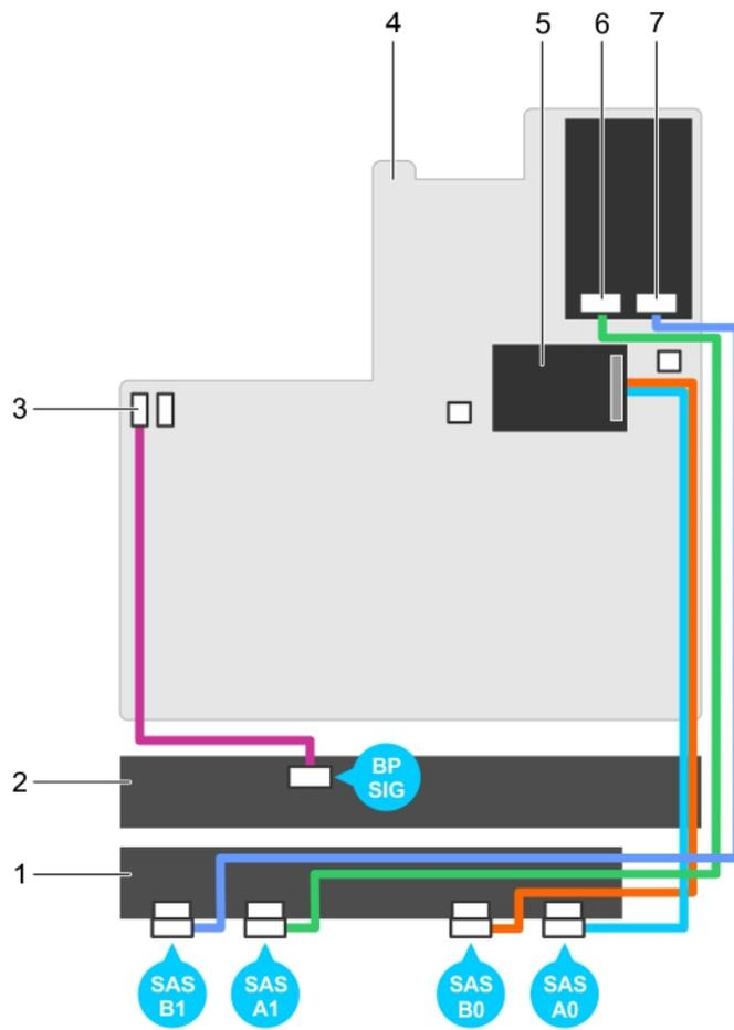
**Figure 56. Cabling diagram—2.5 Inch (x24) SAS/SATA backplane— (option 2)**
