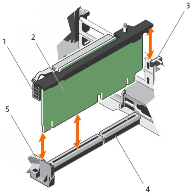
**Figure 36. Removing and installing the expansion card riser 2**
