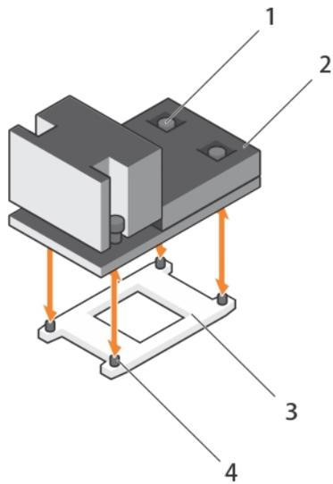
**Figure 22. Removing and installing a processor heat sink**
