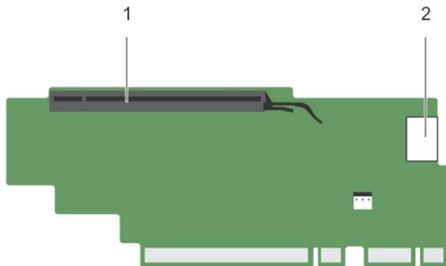
**Figure 40. Identifying connectors on the expansion card riser 3 (alternate)**
