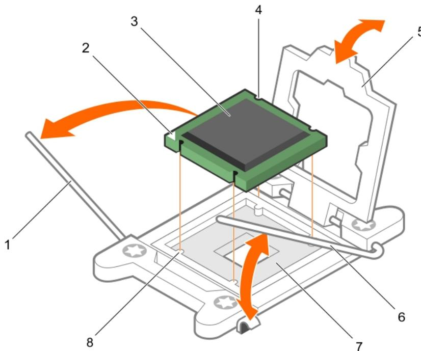
**Figure 25. Removing and installing a processor**
