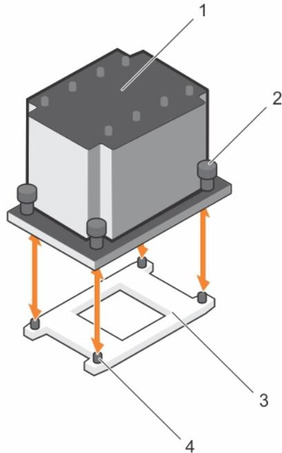
**Figure 21. Removing and installing a processor**
