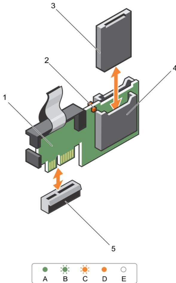
**Figure 41. Removing and installing the Internal Dual SD Module (IDSDM)**
