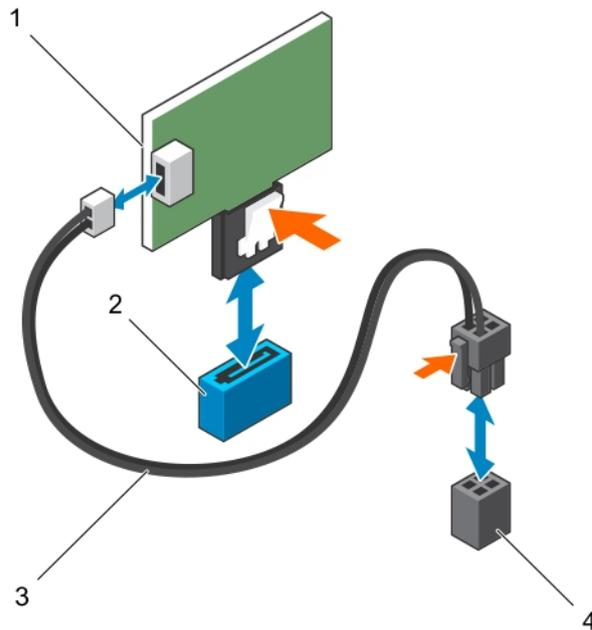
**Figure 20. Removing and installing SATADOM**
