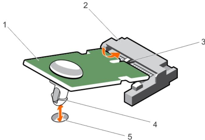
**Figure 49. Installing the TPM**
