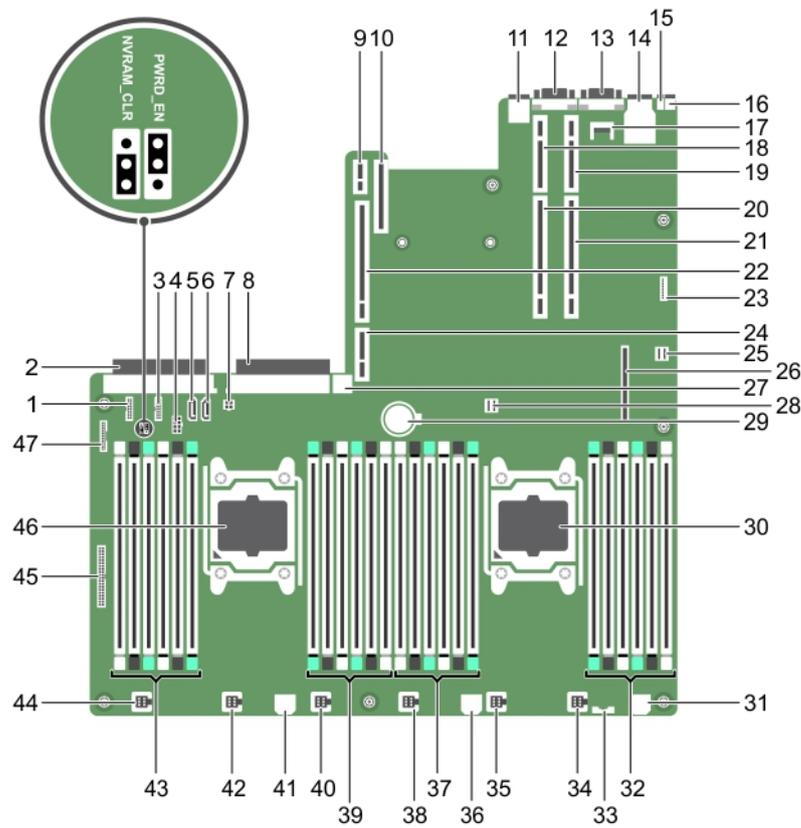
Figure 62. System board jumpers and connectors
