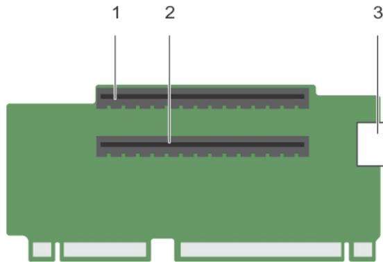
**Figure 37. Identifying connectors on the expansion card riser 2**
