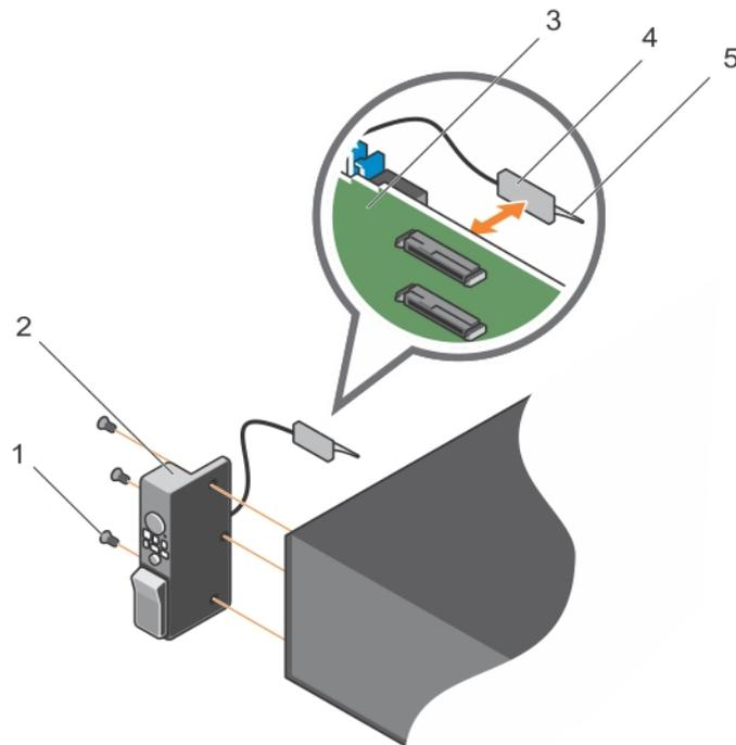
**Figure 59. Removing and installing the control panel**
