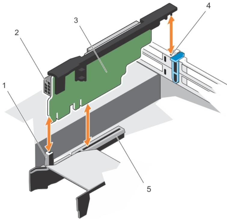
**Figure 38. Removing and installing the expansion card riser 3**
