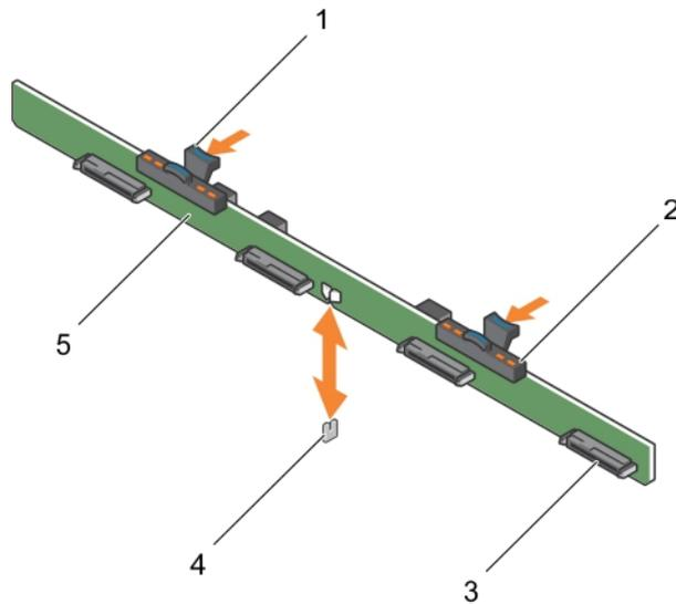
**Figure 61. Removing and installing the 3.5 inch (x4) hard-drive backplane**
