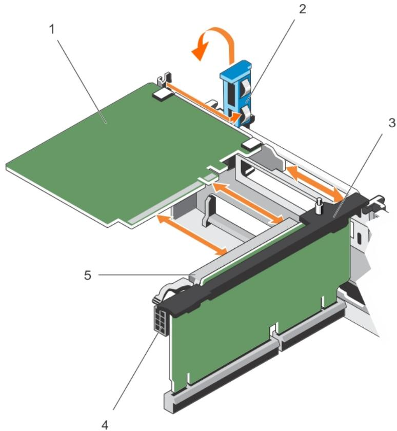
**Figure 32. Removing and installing an expansion card from expansion-card riser 2 or 3**
