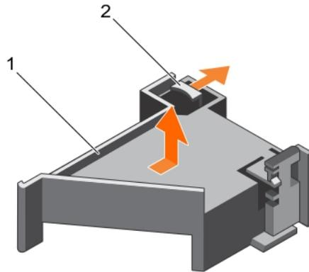
**Figure 27. Removing and installing the PCIe card holder**
