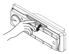
To open the XML8100 and use the dock, pull outward from the top of the front panel.
