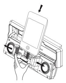
To dock an iPod device, first spread apart the side supports of the dock. Then line up the dock connector and insert the iPod device into the dock. Release the side supports to secure the device.
