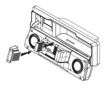
For the 1st generation, 2nd generation and 4th generation iPod Nano devices, the left side dock support can be replaced with a larger rubber support, for the best fit.
