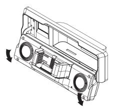
The front panel stops when it reaches the fully open position.
