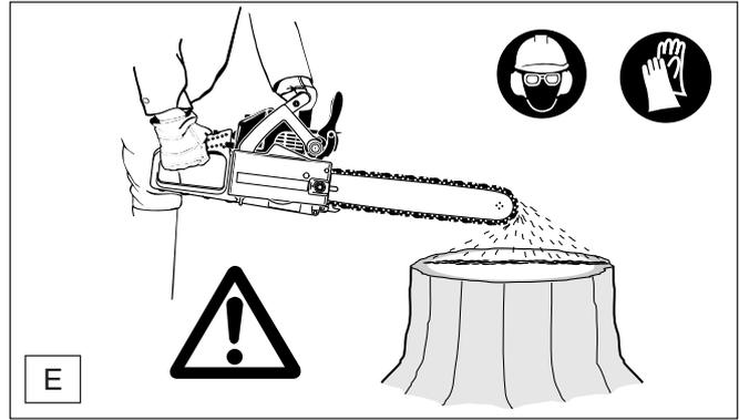
Never work with the chain saw without sufficient chain lubrication. Otherwise the service life of the chain and guide bar will be reduced.
