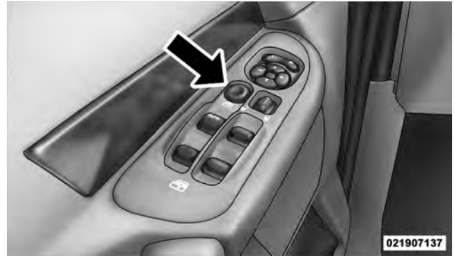
Window Lockout Switch
