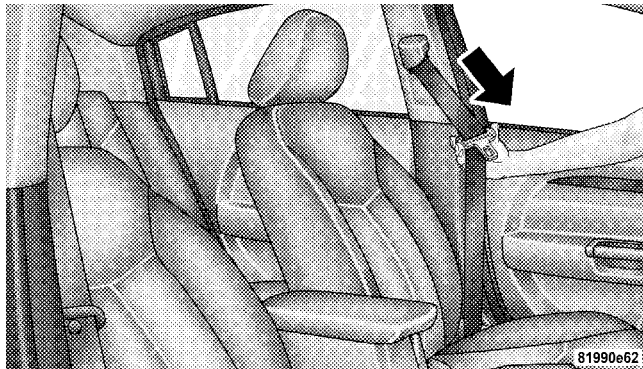
Pulling Out the Latch Plate
