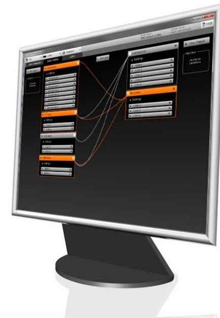
The Audio console helps you configure the audio system of the codec. It will allow you to change the default mixing, routing and equalization as well as allow you to set various input and output connector properties.
