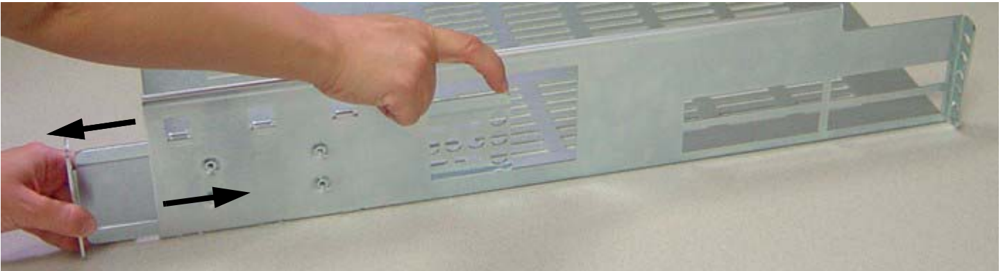
Figure 2-2: Separate the Sliding Bracket From Both Sides of the Shelf Unit
