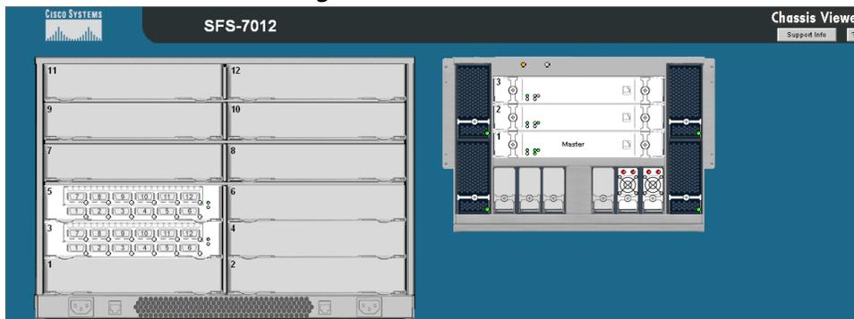
The Chassis Viewer's home page provides a high-level overview of the SFS 7012 switch and individual leaf and spine modules. This area is the starting point to more detailed information for the SFS 7012 chassis and components (fans and power supplies), leaf modules, and spine modules. The selected component provides hyperlinks to related menus and information where the user can perform configuration and monitoring tasks.
