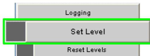
The Set Level button allows the user to set log level configuration parameters for all software modules on the SFS 7012.
