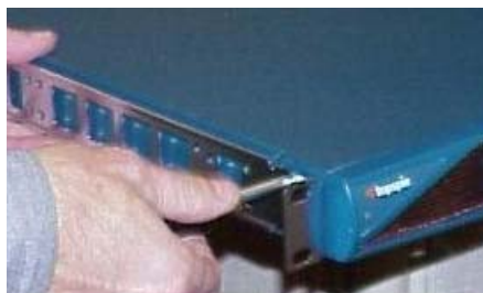
Figure 1-8: Fasten Rack Bracket to Switch Chassis
