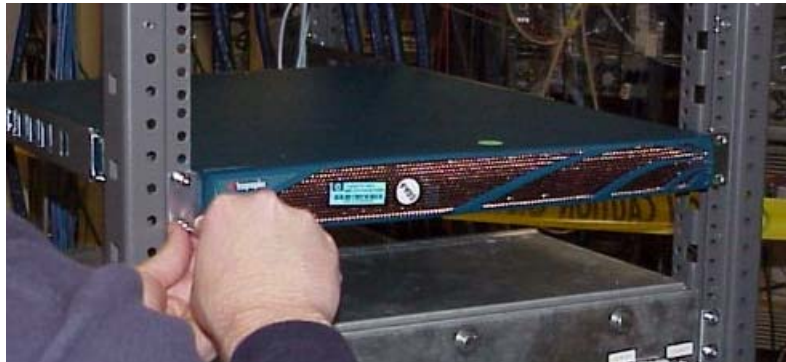
Figure 1-9: Secure the Switch Through the Front Posts
