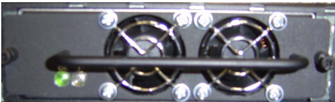
Figure 5-2: Power Supply LEDs
