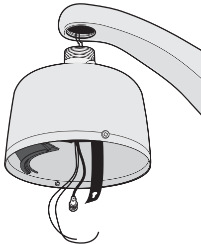
Figure 1-3 Attaching the Pendant Back Box to the Mount
