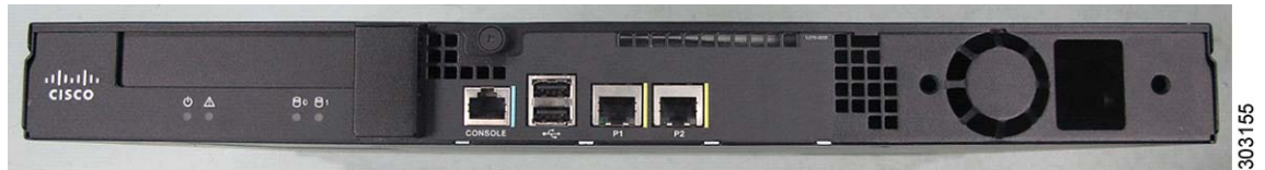
Figure 1-8 Rear Panel and Ports for Cisco C170 and Cisco M170
