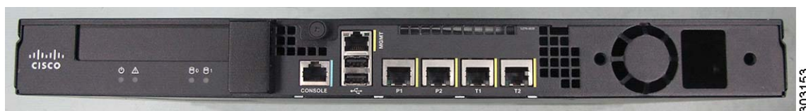
Figure 1-6 Rear Panel and Ports for Cisco S170
