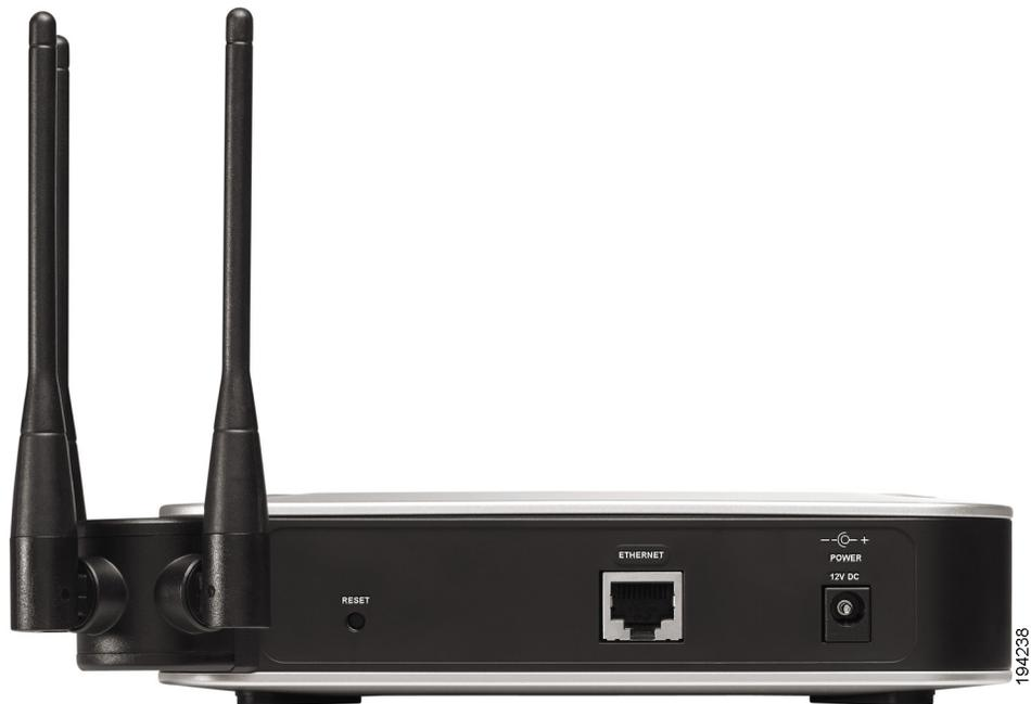
**RESET Button**—There are two ways to reset the access point to the factory default configuration. Either press the Reset button for approximately 10 seconds or restore the defaults using the web-based utility of the access point.
