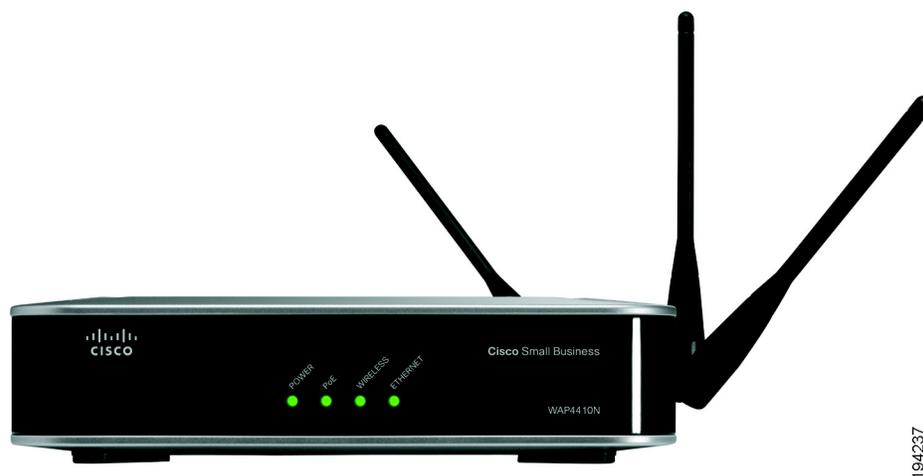
The access point's front panel LEDs display information about network activity.
