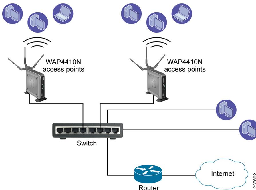
The wireless access points are connecting to a Cisco switch that provides them with power. Each access point can connect multiple wireless devices to the network.
