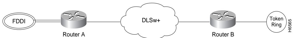
Figure 136 DLSw+ Translation Between FDDI and Token Ring
