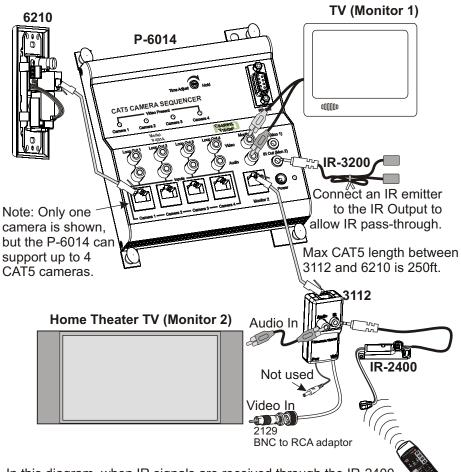
In this diagram, when IR signals are received through the IR-2400 they are sent back to the P-6014 through the 3112. These IR signals will only affect the Monitor 2 output. The Monitor 1 output can be independently controlled by connecting an IR receiver to the "IR Input" jack on the P-6014.
