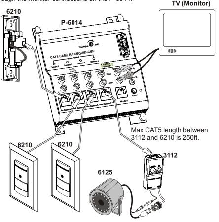
The P-6014 can be used with Channel Vision's 6210 CAT5 camera or any conventional camera when used with the 3112 accessory. The 3112 has multiple applications, but when used in this application the IR connection will not be used and the Audio connection would only be used if your conventional camera has a built-in microphone.
