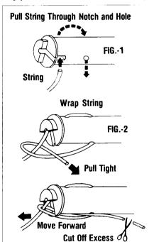
2. As shown in FIG-1 above, strings pass through a notch in the end of the sensor, and then through a hole in the sensor. After pulling through a few inches of string, tie the string as shown in FIG-2. Next, fix the string tight and cut off any excess.
