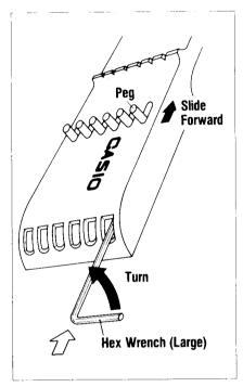
3. Insert the accessory hex wrench (large) into the head and turn it counter-clockwise to slide the headpiece towards the body. Next, insert the other hex wrench (small) in the headpiece and loosen the screw.
