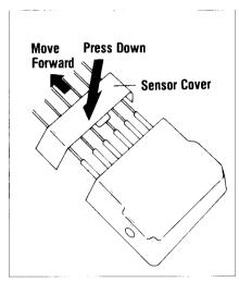
1. As shown in the above diagram, press down on the sensor cover and move it toward the neck.
