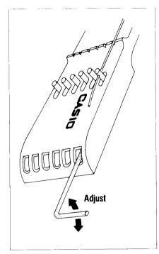
4. Next, pull the string through the hole in the headpiece and tighten the headpiece screw while pulling the string taut.
