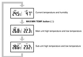
• To clear the high temperature and low temperature data memory, press the **CLEAR button** ((§)). New data starts to be stored after memory is cleared.
