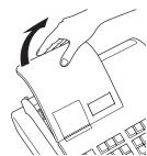
**2** Remove the battery compartment cover.
