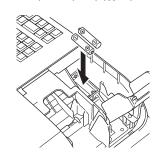
**4** Replace the battery compartment cover and the printer cover.
