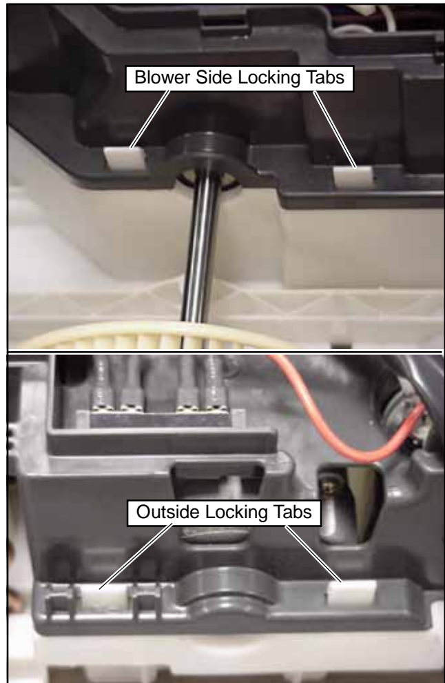
Figure 3-34 Evaporator Motor Locking Tabs
