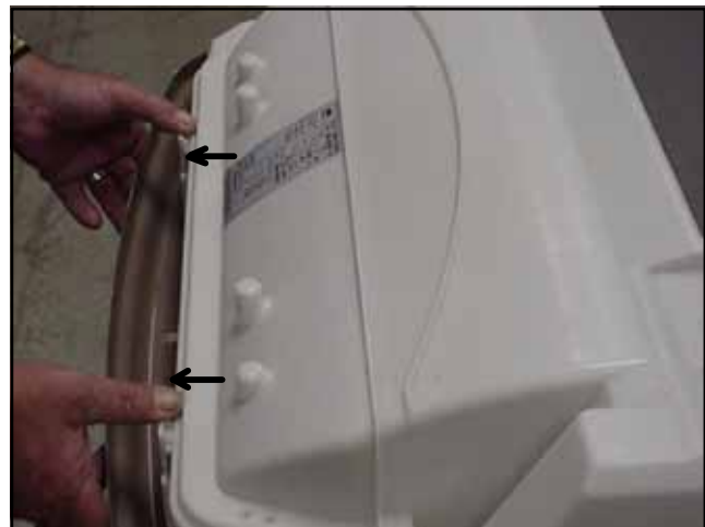
Figure 3-28 Upper Scroll Assembly Keeper Tab Release
