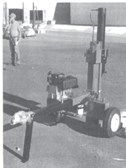
Beam attached to tank/tongue assembly (see step 8, pg. 8).
