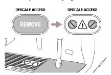
b) Use a flat-head screwdriver to rotate the right screw counter-clockwise until the valve is fully open. As the valve opens, steam may be released. When the water is completely empty, close the valve by rotating screws clock-wise until seated. Do not overtighten screws to avoid damages to the valves.
