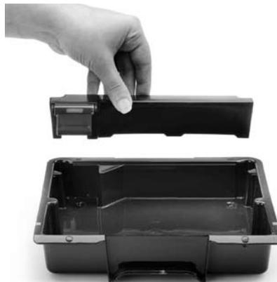
Insert the 'Empty Me!' full indicator into position in the drip tray and place the stainless steel grid on top. Slide the drip tray into position in the base of the machine in front of the storage tray.
