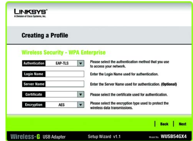
Figure 5-27: Wireless Security - WPA Enterprise Using EAP-TLS Screen
