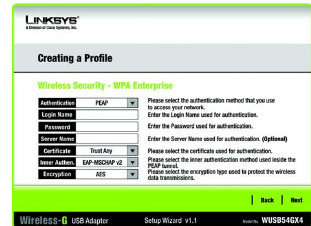
Figure 5-28: Wireless Security - WPA Enterprise Using PEAP Screen
