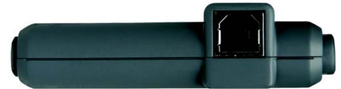
Figure 3-1: USB Network Adapter's USB Port
