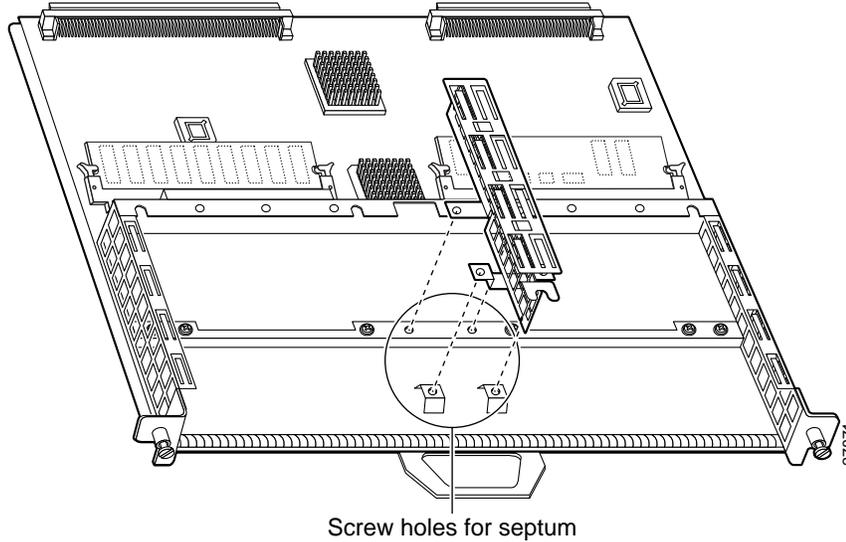
Use the following procedure to remove the slot divider from a VIP4:
