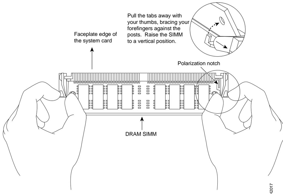
**Step 6** Using the SIMM orientation shown in Figure 12, position the new SIMM so that the polarization notch is located at the right end of the SIMM socket.
