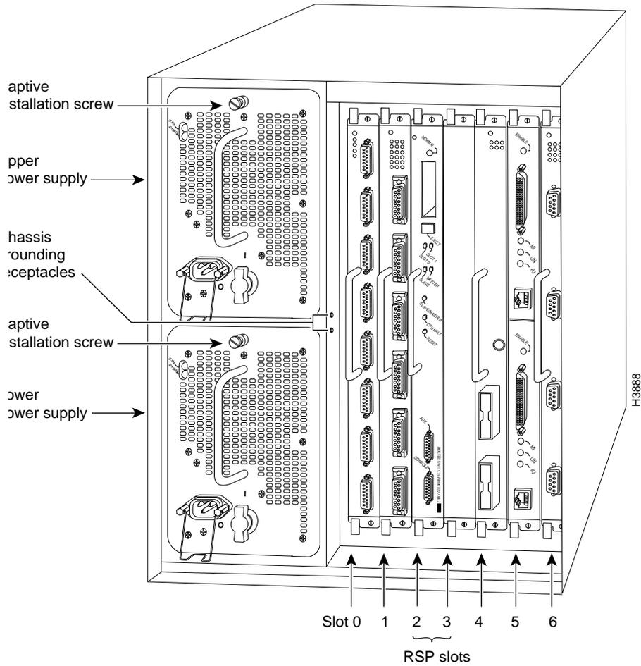
Figure 6 shows the rear of the Cisco 7513 with two AC-input power supplies installed. Two slots (6 and 7) are reserved for the second generation Route Switch Processor (RSP2), which contains the system processor and performs packet switching functions. Slots 0 through 5 and 8 through 12 are for interface processors.
