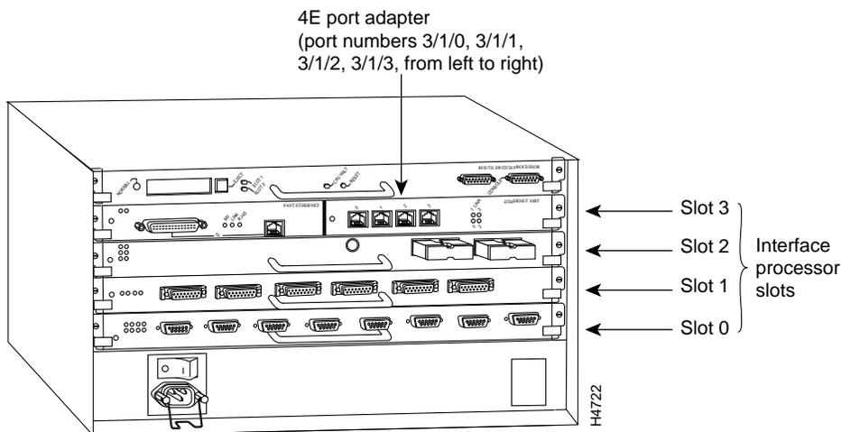
**Note** VIP configurations using only one 4E port adapter, and a port adapter blank, or two 4E port adapters, are currently not supported.
