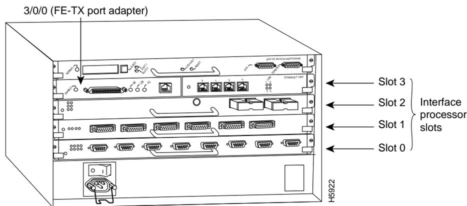
**Note:** The MII and RJ-45 interface ports on the first port adapter are both numbered as interface port 0. Only one of them can be used on each port adapter, at one time.
