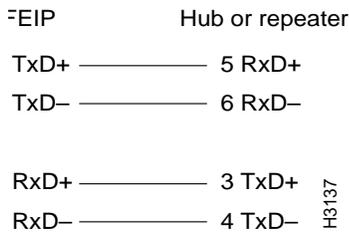
**Figure 28 Crossover Cable Pinout, 4E RJ-45 Connections Between Hubs and Repeaters**
