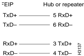
**Figure 18 Crossover Cable Pinout, FE-TX RJ-45 Connections between Hubs and Repeaters**
