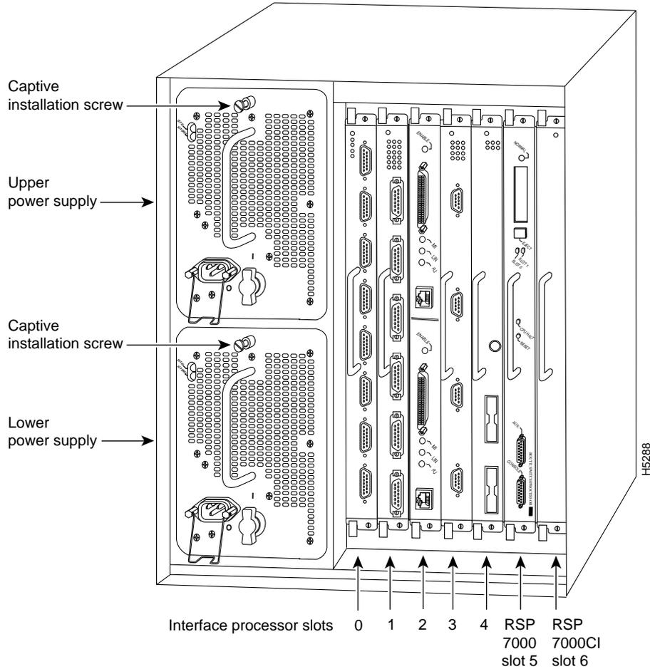
**Figure 3 Cisco 7010, Interface Processor End**
