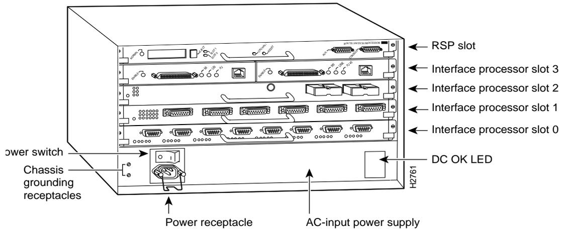
Figure 5 shows the rear of the seven-slot Cisco 7507 router. In the Cisco 7507, up to two slots (2 and 3) are reserved for the Route Switch Processor (RSP), which contains the system processor and performs packet switching functions. Slots 0 and 1 and 4 through 6 are for interface processors.
