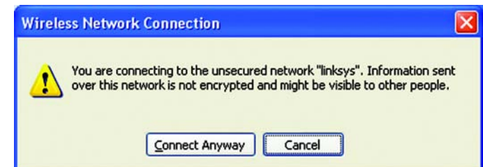
Figure B-5: No Wireless Security
