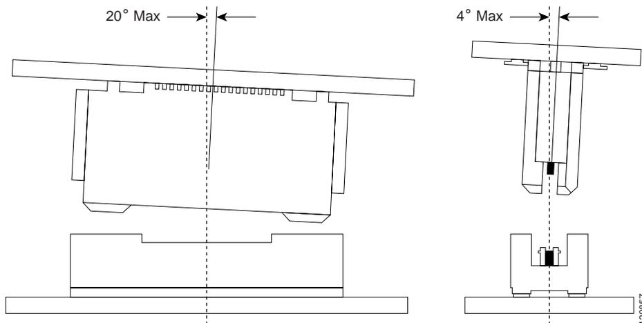
**Step 3** Ensure that the connector guide pins are aligned. Once the connector is engaged, apply gentle pressure with your thumbs to the two rear outer corners of the EPA, as shown in [Figure 11](#) and [Figure 12](#).
