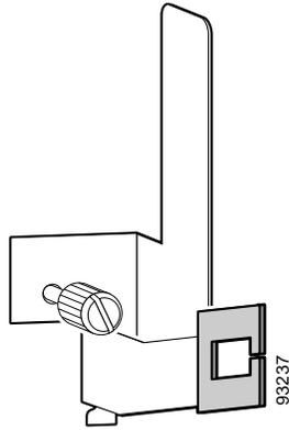
**Figure 31** *Multiport Line Card Cable-Management Bracket*
