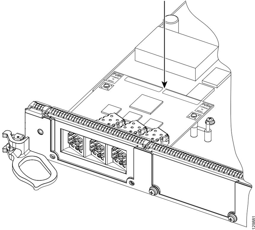
**Step 5** Use a Phillips screwdriver to insert and tighten the screw on the EPA, 3 to 5 in-lbs, as shown in [Figure 14](#).
