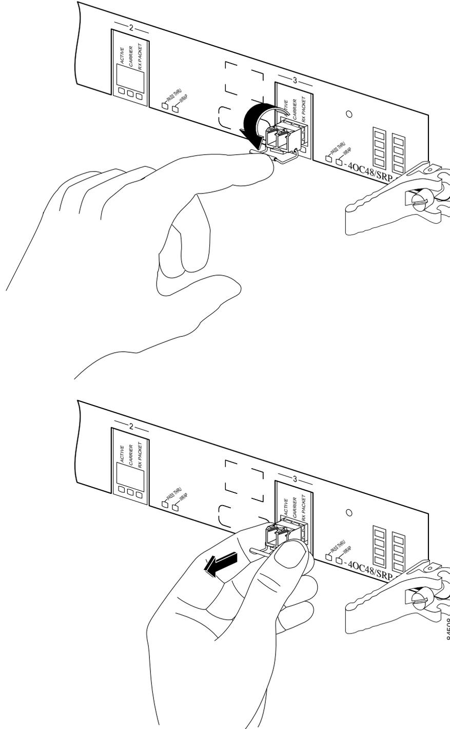
**Step 5** Place the removed SFP module on an antistatic mat, or immediately place it in a static shielding bag if you plan to return it to the factory.
