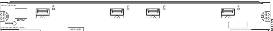
There is one line card Status LED and two port Status LEDs. [Table 2-3](#) provides LED descriptions.
