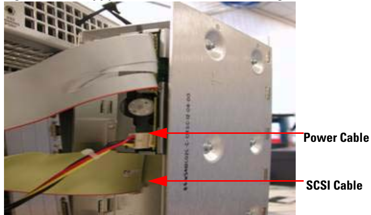
Figure 2 Floppy Disk Drive Inside the Housing
