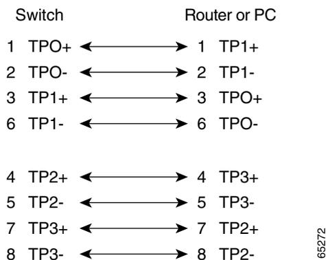
**Figure A-8 Four Twisted-Pair Crossover Cable Schematics for 10/100/1000 Ports**
