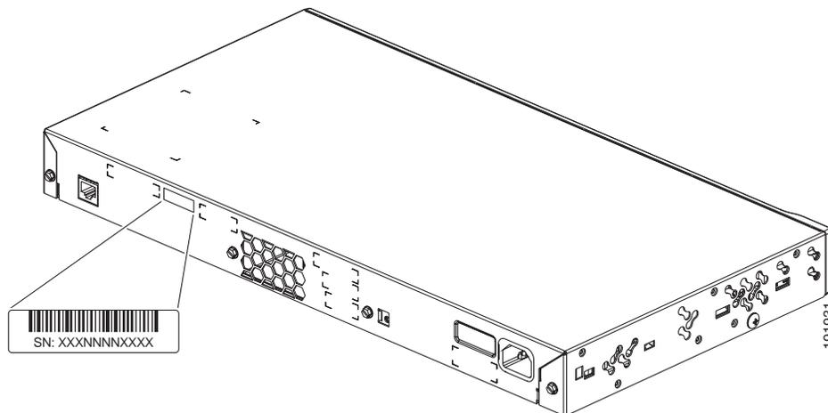
**Figure 4-3** Serial Number Location on the Catalyst 2960-8TC-L, Catalyst 2960G-8TC-L, and Catalyst 2960PD-8TT-L Switches
