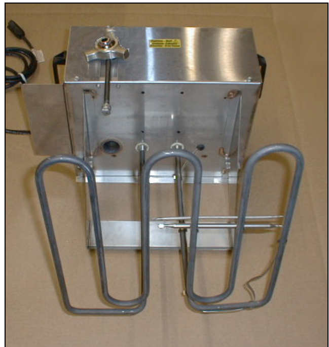
Figure 3-1. Removing the Heater Head. (Place heater head as shown above so no damage is done to the element.)
