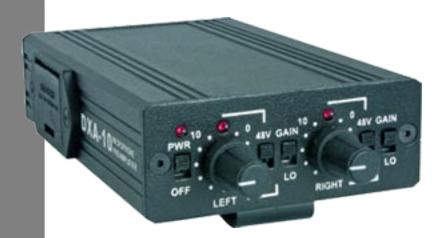
The BeachTek DXA-10 is a two channel, battery-powered microphone preamplifier with built in dual phantom power. This device is ideal as a very quiet front end for the Sony FX1 camcorder. Can also be used as a general purpose XLR microphone to line level amplifier. The DXA-10 gives you studio quality audio in portable, battery operated unit.
